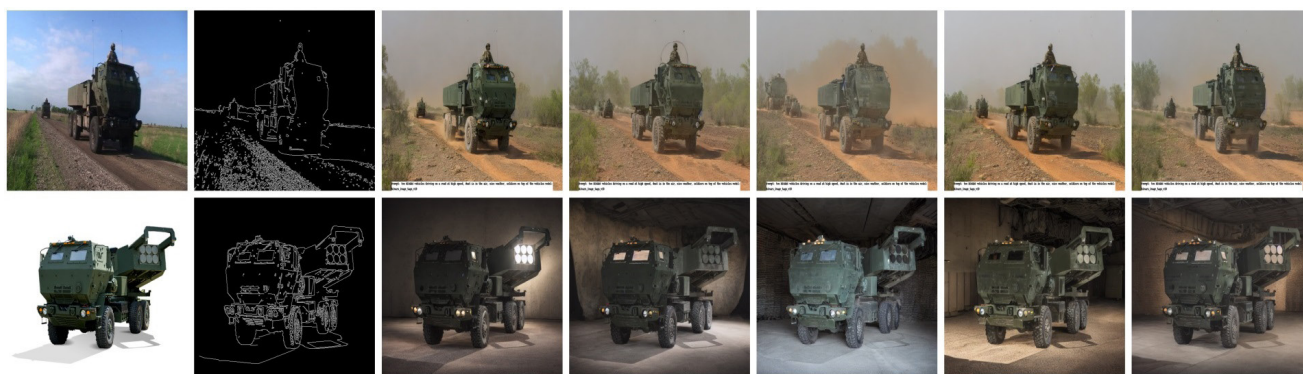
Synthetic image generation with Stable Diffusion using the example of a HIMARS guided missile launcher. From left to right: Original image, canny-edge map, five different synthetic examples. The canny-edge map is used as input for Stable Diffusion and guarantees that the geometry of the vehicle is preserved as far as possible. Stable Diffusion can now change the original image such that the vehicle appears in a different environment than in the original image. In future, threat players could use such a method in combination with a targeted distribution over social media for the purpose of military deception.
