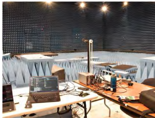
Experimental set-up in the lab in order to take over drones in a controlled environment via GPS spoofing.
