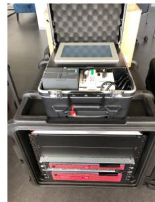
Industrial control system with a visualization display (top) and a mobile cyber section (bottom)
